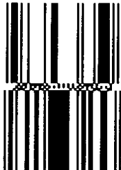
RSS-14 Stacked Omnidirectional
